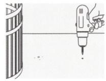
**3.** Set unit aside. Using power drill and concrete bit to 7/16" holes into the concrete. Depth of holes should be  $2\frac{1}{2}$ ".
