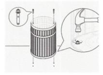
4. Align unit over the holes and insert supplied wedge bolts (supplied with base, taped to the liner handle) through unit into holes in concrete. Tap down as necessary and tighten.
