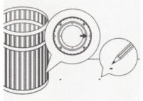
MOUNTING TO CONCRETE: Use pencil to trace and mark locations on concrete of mounting holes on bottom of unit.
