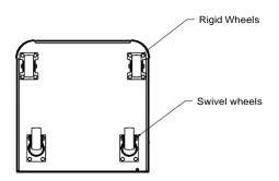
Lay the unit on its side and attach the 4 casters with the 16-- 1/4-20 hex bolts.
